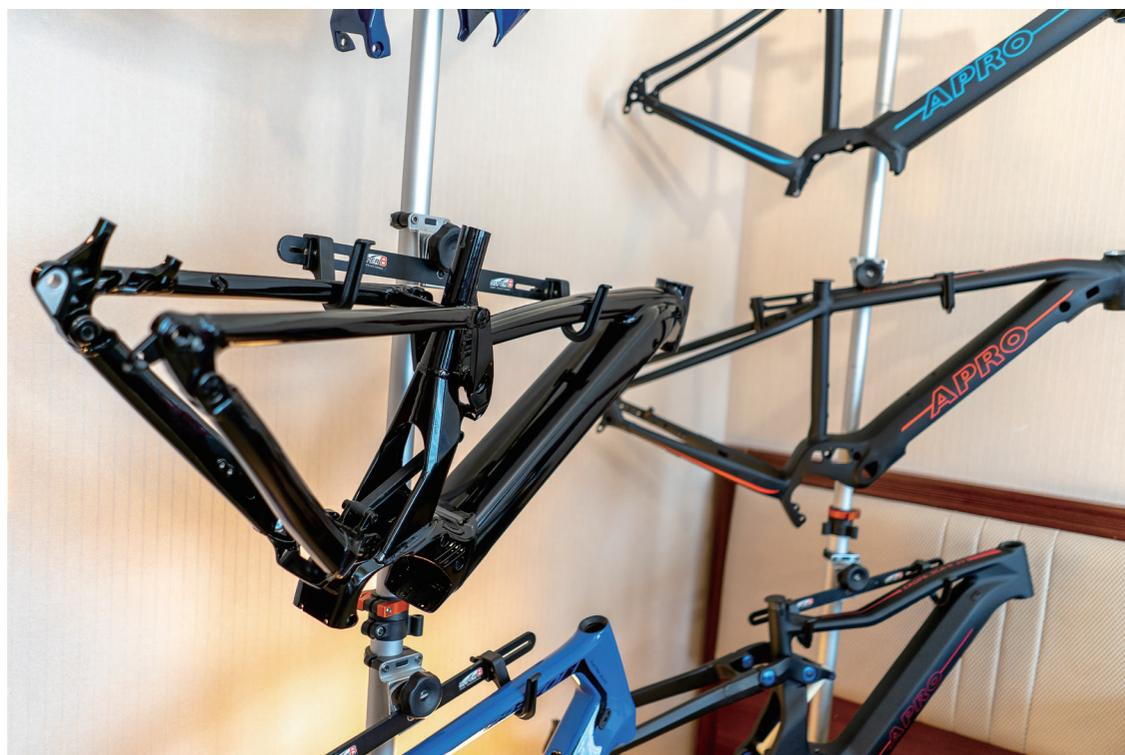
▲ Apro's ERDP6.0A-B29 e-bike frame features an RDP design allowing for increased pedaling efficiency.
