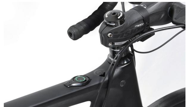
▲ The System features an integrated on-bike control.
